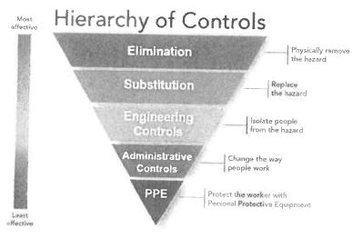
The idea behind this hierarchy is that the control methods at the top of graphic are potentially more effective and protective than those at the bottom. Following this hierarchy normally leads to the implementation of inherently safer systems, where the risk of illness or injury has been substantially reduced.
